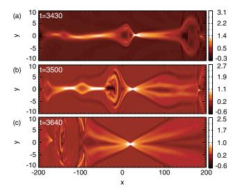
FIG. 3 (color). Time evolution of  $J_z$  from the other current sheet in our double tearing mode setup, showing the ejection of secondary islands when Hall reconnection onsets.
