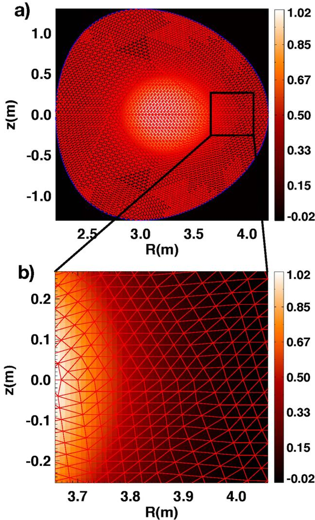
**Figure 2.** (a) View of the toroidal current density at a constant toroidal angle over-plotted with the triangular finite element mesh. (b) Zoomed in portion of the domain in (a) to show the resolution of the mesh, with an average edge length of 0.04 m.
